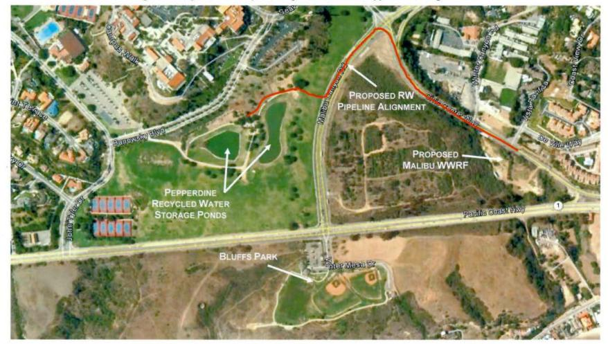
Figure 5: Recycled Water Pipeline Alignment to Serve Pepperdine Storage Ponds
